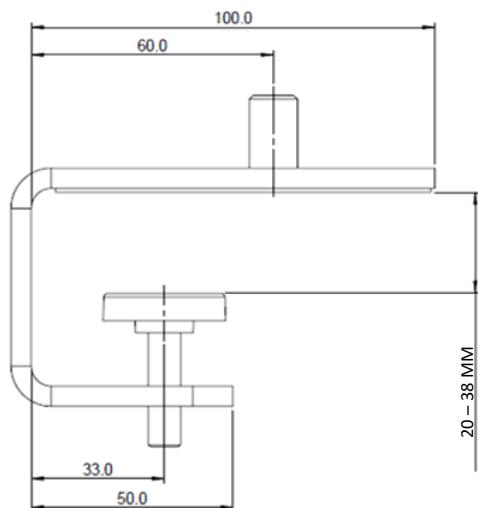
\*Note that dimensions provided are measured in mm
